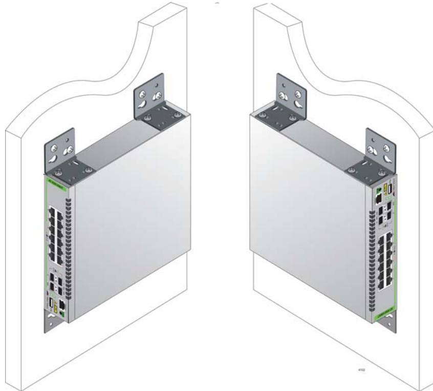
Figure 32. Positioning the Switch on the Wall
