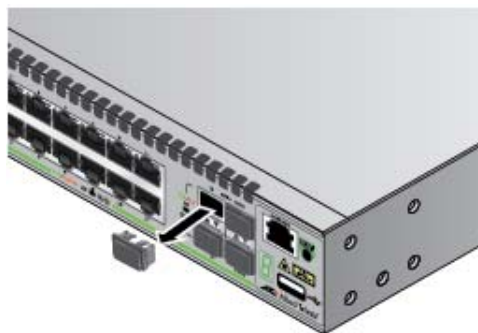
Figure 39. Removing the Dust Plug from an SFP/SFP+ Slot
